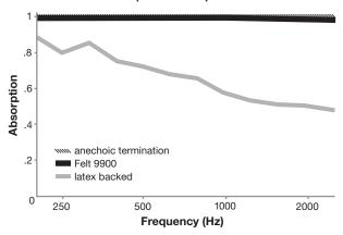
NRC of anechoic termination 1.00 NRC of fabric in front of anechoic termination 0.99
