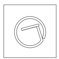
SM-Clip fully engaged, top view
