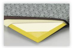
CORE Facing: Perforated .060 co-polymer Backing: 6-7 pcf fiberglass, 1"-4" thick
