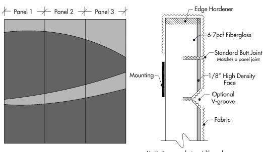
Limitations apply to width and depth of optional v-grooves
