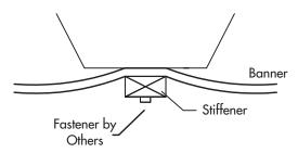
Stiffeners are attached at both ends. An intermediate stiffener is attached at the mid-point of Banners longer than 120". Intermediate stiffeners are shipped loose and attached in the field.
